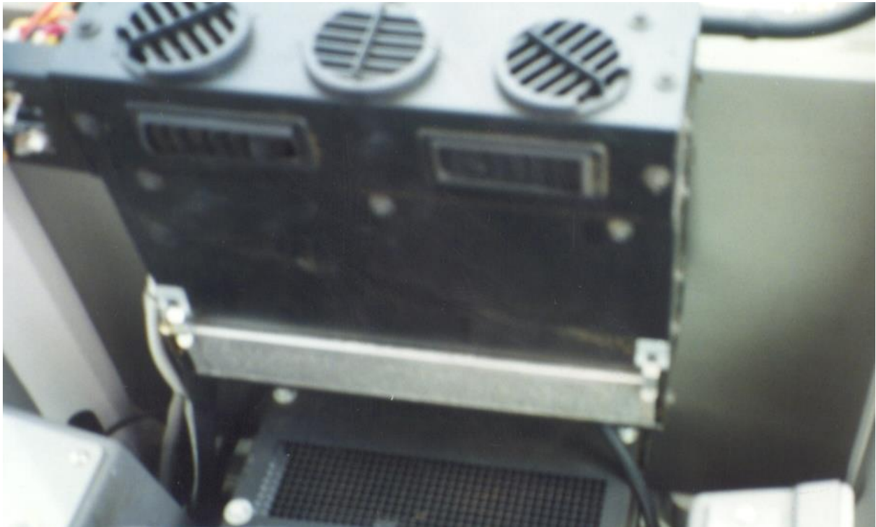
Evaporator assembly mounted in place.
